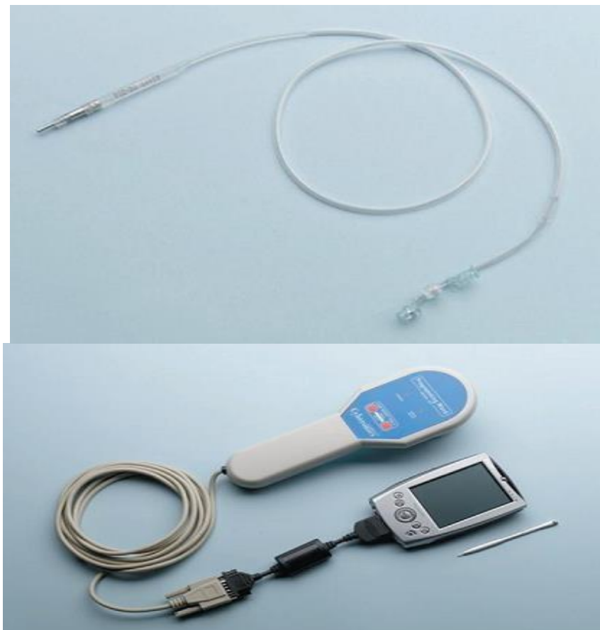
Fig. 4 shows the programming wand for vagal nerve stimulation, along with the programming computer, which is of the personal digital assistant type. [24]
