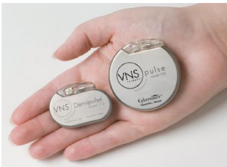
Figure 2. Side views of vagal nerve stimulation devices, demonstrating a steady reduction in size from the original model 100 generator in 1994 to the current model 103/104 generator (2007). [24]
