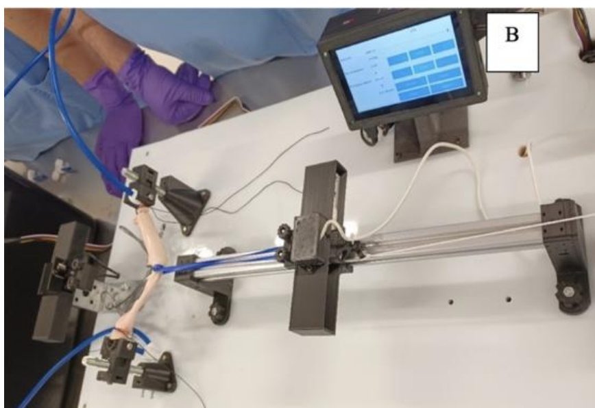
Figure 3 — Laboratory Setup for Vascular Tissue Testing
