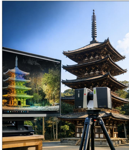
3D laser scanning and digital documentation of a historic Japanese pagoda.
