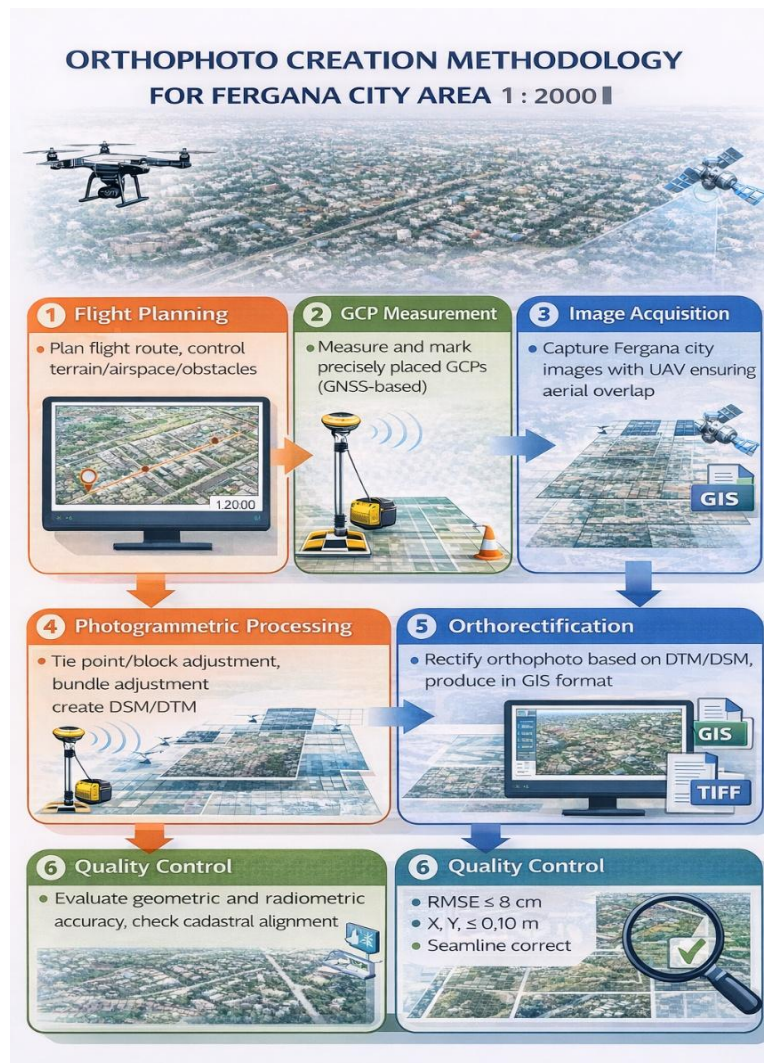
Figure 2. Methodology for creating and assessing the quality of an orthophotomap based on UAV photogrammetry for the Fergana city area
